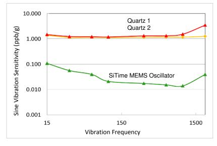
Vibration resistance is important since electronic systems are often exposed to environmental stresses, especially systems deployed outdoors. Wind, heavy vehicles and trains are a few examples of the many sources of external vibration. In addition, systems often employ cooling fans that cause vibration. These vibration stresses can induce frequency shift and noise on the crystal resonator.
