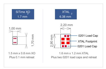
Oscillators are a completely integrated solution and do not require external components such as power supply decoupling caps. SiTime's 1.5 mm x 0.8 mm (1508) footprint is smaller than the smallest quartz crystal footprint at 1.6 mm x 1.2 mm. And when taking into account load capacitors that are needed for the 32 kHz quartz crystal, the total board area or the XTAL solution is over three times larger.
