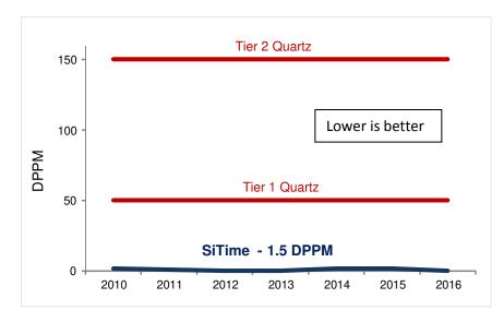
As a result, the DPPM and MTBF of SiTime oscillators are about 30 times better than quartz, providing a very reliable technology platform that endures severe environmental stresses and delivers a high quality product for the end user.
