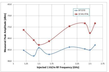
This test was performed per IEC 62132-2 standard that injects electromagnetic energy into a transverse electromagnetic (TEM) cell where the device under test (DUT) is mounted.
