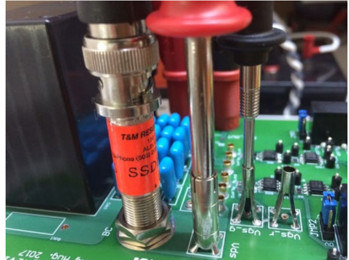
Figure 8: Probe-tip to PCB interface connections
