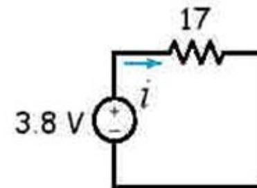
step #4: circuit after combining the two sources and the series resistors.
