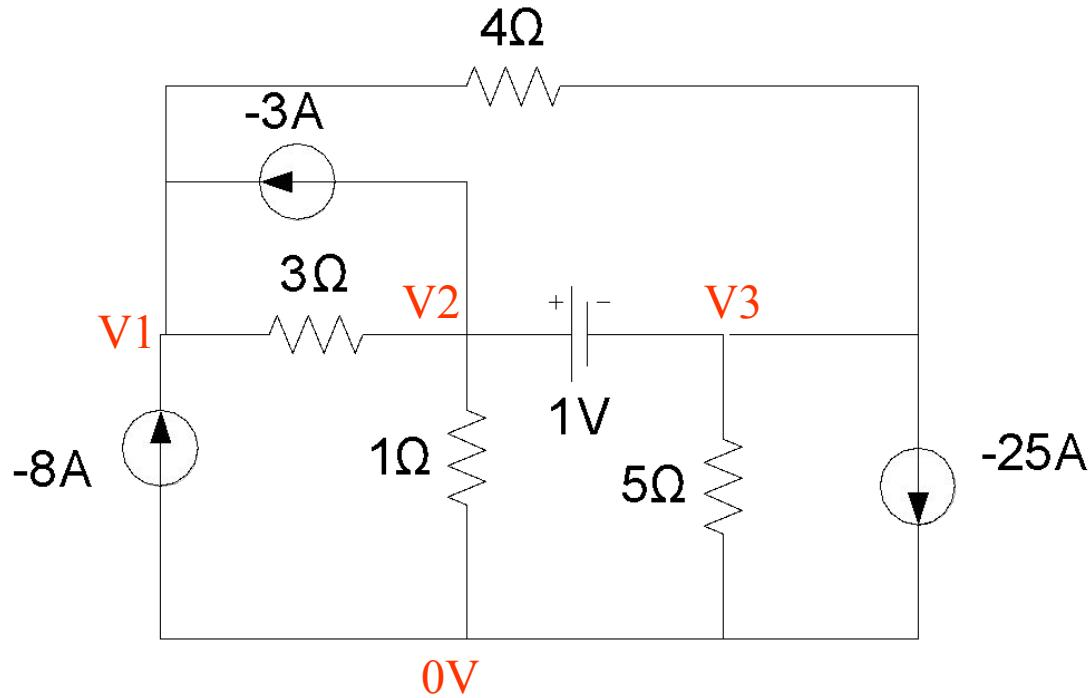
$$8 + \frac{V_1 - V_3}{4} + 3 + \frac{V_1 - V_2}{3} = 0$$
