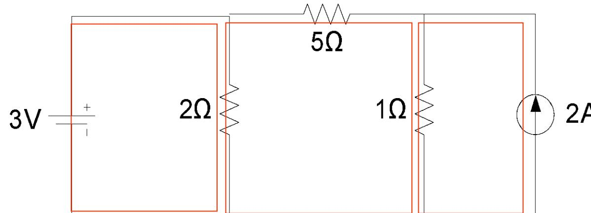
Mesh currents are circular currents used for calculation.
