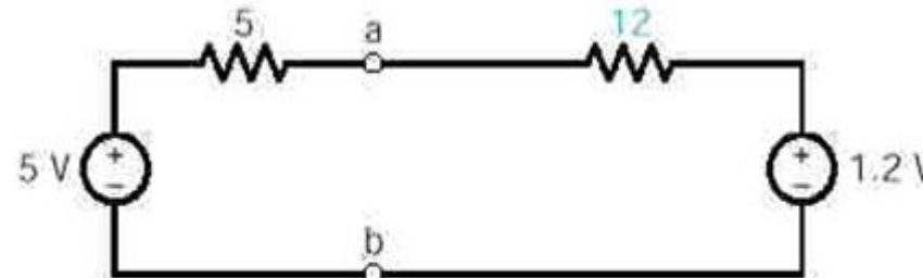
step #3: circuit after transforming the 0.1 A source
