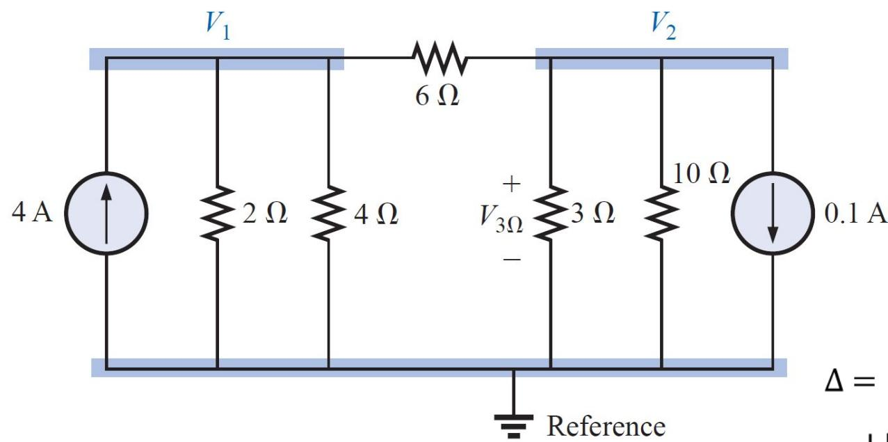
$$\left. \begin{array}{l} \left( \frac{1}{2\Omega} + \frac{1}{4\Omega} + \frac{1}{6\Omega} \right) V_1 - \left( \frac{1}{6\Omega} \right) V_2 = +4 \text{ A} \\ \left( \frac{1}{10\Omega} + \frac{1}{3\Omega} + \frac{1}{6\Omega} \right) V_2 - \left( \frac{1}{6\Omega} \right) V_1 = -0.1 \text{ A} \end{array} \right\}$$
